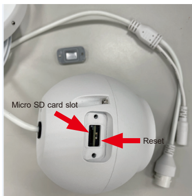
Figure 5-3: Reset Button and micro SD card slot of ICA-M4580P
